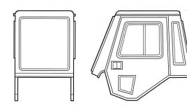
**Steel Cab** enclosure with high visibility safety glazing that replaces the existing factory overhead guard.
